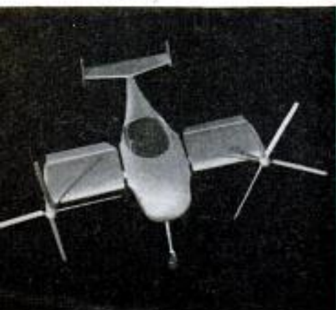
Single rear engine drives rotors of a pivoting-wing Convertawing
